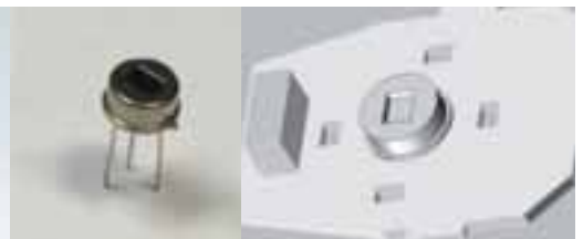
Human Activity Sensor Detects human movements, changes in activity levels and human absence.
